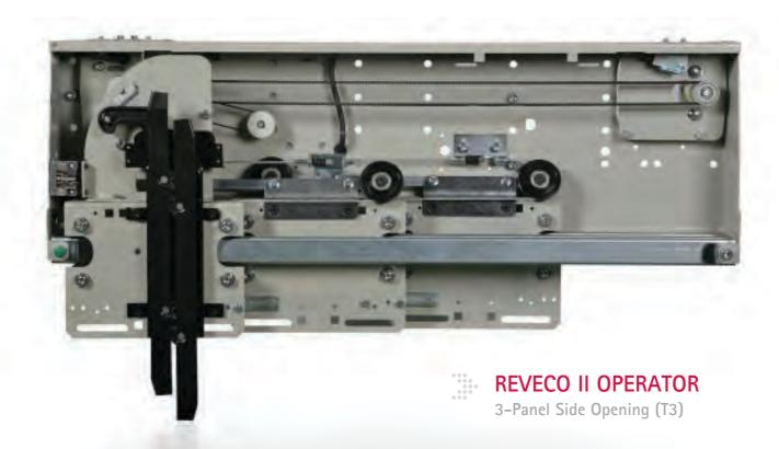
3-panel side-opening car door operator, supplied with 230 Vac singlephase voltage. It is controlled by an electronic system enabling speed regulation through 3VF frequency variation/voltage variation. Reading of door speed, position and direction of movement is carried out through double pulse encoder, integrated with the electronic circuit. There are no positioning microswitches
