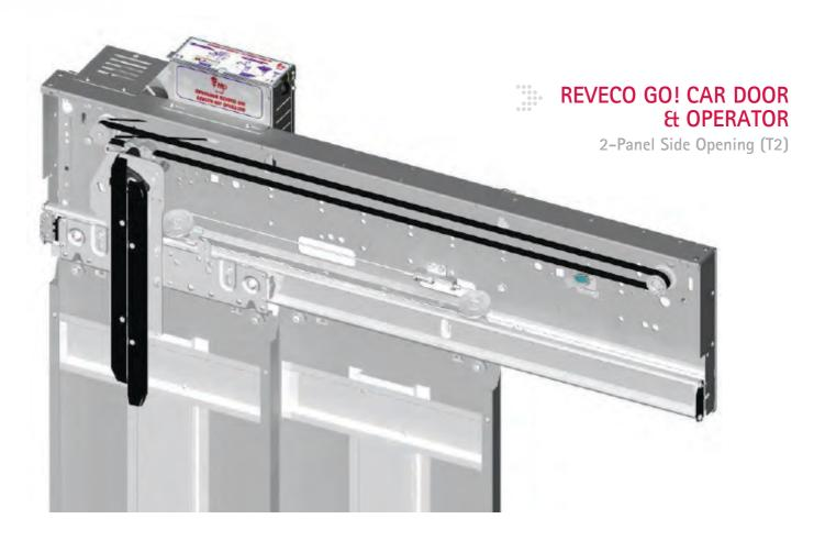
Two-panel side opening car door operator, powered by single-phase voltage of 230 Vac. It is controlled by an electronic system (3VF) which adjusts speed by means of frequency variation voltage regulation. Reading of door speed, position and direction of movement is carried out through a double pulse encoder, which is integrated into the electronic circuit. There are no positioning microswitches
